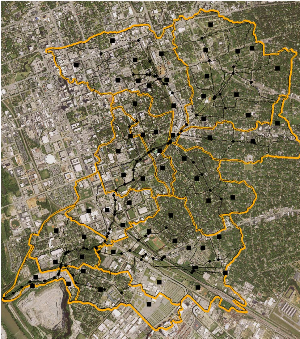
Figure 2.4. SWMM Model Layout including all subcatchments, links, and nodes. Only the upper portion of the model above Pickens was calibrated and used for this study
